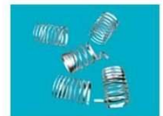
Loosely rolled chips indicate Optimum cutting conditions.
