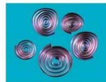
Thick, heavy or blue colored chips indicate that the saw blade is being overloaded.
