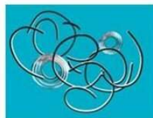
Very fine pulverized chips. Feed speed should be increased.
