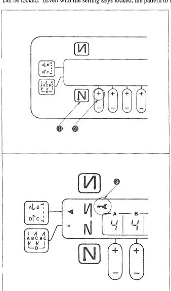
1) After the completion of the setting of data on the number of stitches, etc., turn OFF the power to the machine once.
