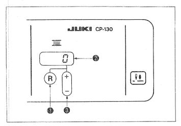
1) Press bobbin thread counter reset switch (1) to return the value indicated on bobbin thread counter (2) to the initial value (it has been factory-set to "0" at the time of delivery).
