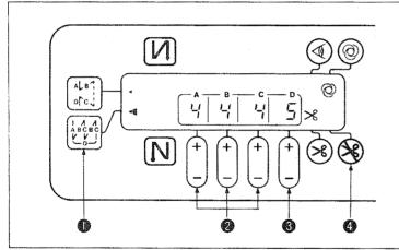
1) Press overlapped stitching pattern switch • to specify the overlapped stitching pattern.
