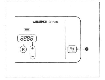
Every time needle up/down compensation switch is pressed, the needle goes up when it is in its lowest position or comes down when it is in its highest position. This compensates the stitch by a half of the predetermined stitch length.
