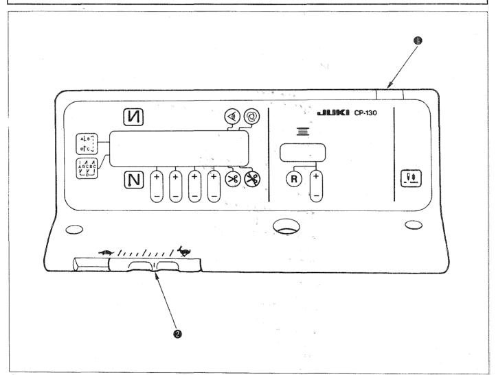
Power indicator lamp (LED): Lights up when the power switch is turned ON.
