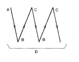
3) If you want to change the number of stitches, operate the "+" or "-" switch of switches of for setting the number of stitches for processes A through C. If you want to change the number of whole processes, operate the "+" or "-" switch of switch of for setting the number of processes D.
