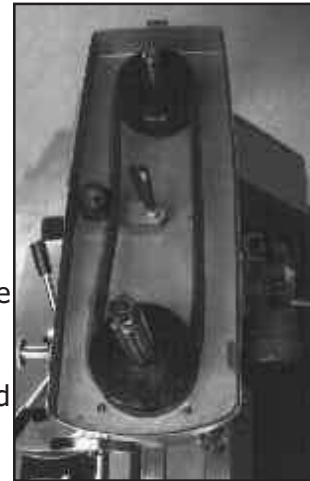
Figure 5.28 Adjusting Millhead Belt Tension
