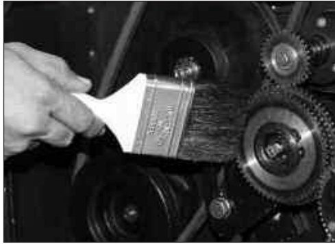
Figure 5.5 Brush a thin layer of lithium grease over the gear quadrant in the pulley box
