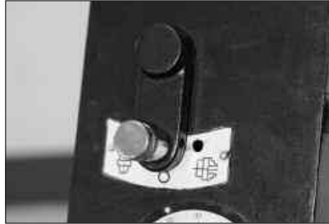
Figure 7.1 Lathe/Mill Clutch Shown in the Neutral Position
