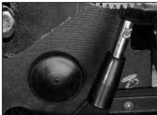
Figure 10.4 Inch/metric Selector located inside the pulley box
