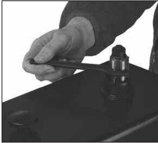
Figure 6.5 Use the supplied spanner wrench to hold the spindle in place while tightening the drawbar
