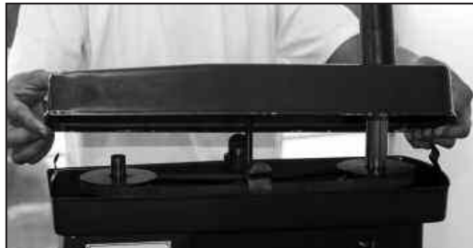
Figure 5.3 Installing Mill Spindle Cover
