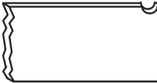
Figure A.7 A crater starts the chip curling smoothly
