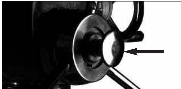
Figure 7.3 Mill/Drill Clutch pushed in engaging the Fine Feed
