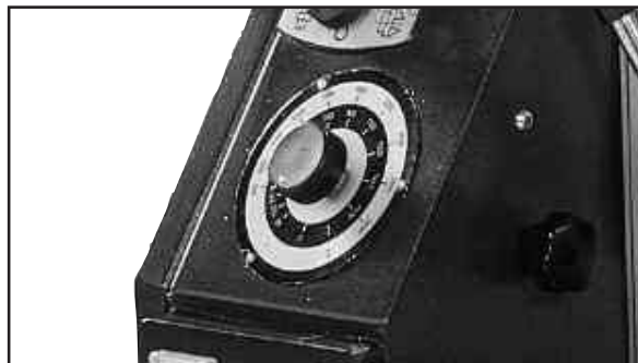
Figure 8.1 Use the Granite Speed Dial for fine adjustments
