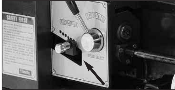
Figure 5.14 Oil the Quick Change Gear Box through the Powerfeed Slot
