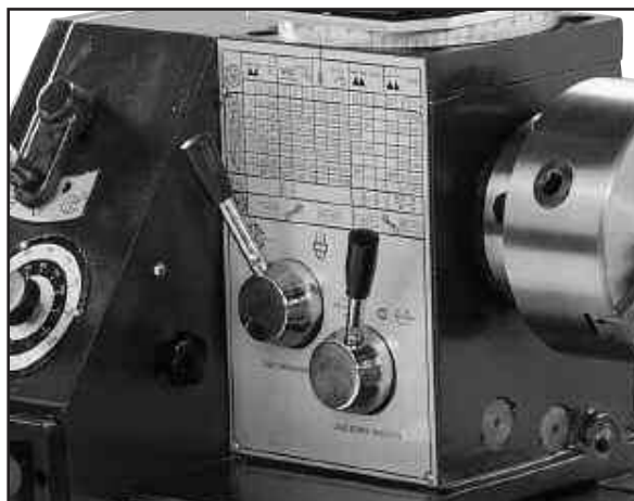
Figure 9.1 Always match the Powerfeed Function lever to the appropriate operation
