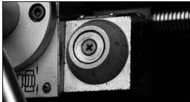
Figure 10.6 Note the number on the threading dial as your halfnut engages
