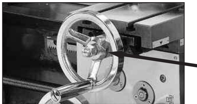
Figure 5.21 Loosen the two outer nuts holding the handwheel
